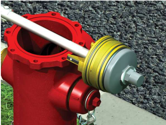
(11) Reassemble the valve components according to the order in which they were disassembled. The valve bottom plate nut (#49) must be tightened to approx. 100 ft-lb. Bend the lock washer (#48) over one edge of the valve bottom plate and over an opposite edge of the valve bottom plate nut.
