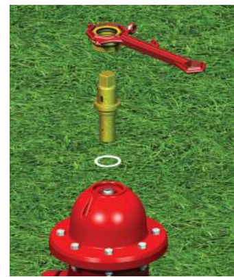
(15) Reinstall the operating nut and anti-friction washer. Before installing the hold down nut, inspect the o-ring and replace if cracked or split. Apply some FIREFLO Lubricant to the o-ring and install the hold down nut. Tighten the hold down nut and the bonnet bolts and nuts.
