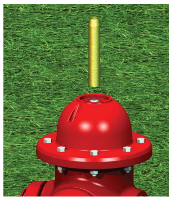
(14) Unthread and remove the brass sleeve from the upper rod and bonnet.
