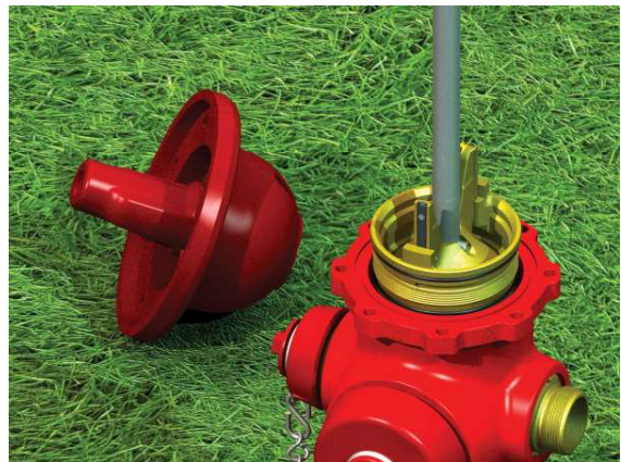
(12) After reassembling the valve components, replace the rod assembly by lowering it into the hydrant barrel. Take caution not to damage the o-rings while lowering the assembly. Use the seat wrench and seat wrench flange to tighten the rod assembly to 375 ft-lb.
