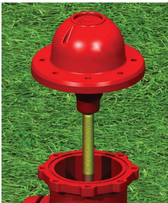
(13) Apply some FIREFLO Lubricant to the bonnet o-ring and install it into the flange groove of the upper standpipe. Check for appropriate lubrication and thread the brass sleeve onto the upper rod and reinstall the bonnet and bonnet bolts without fully tightening.
